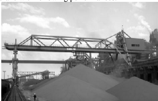
Figure 14. RGP crane; Q = 320 \text{ kN} , 76,2+31,8+6 \text{ m} ; Manufacturer GOŠA
