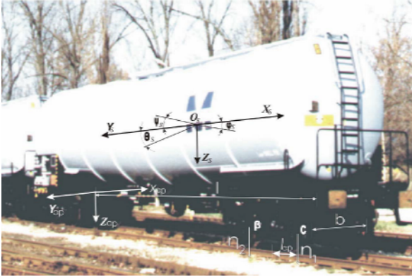
Figure 1 System of coordinate axes of a wagon
