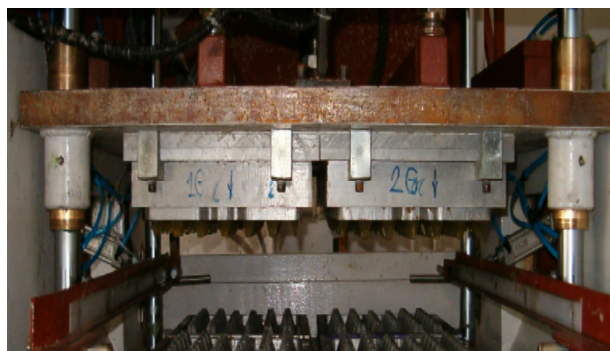
Fig.9 Middle plate with transfer tools as part of forming machine
