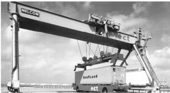
Figure 8. Fully automated gantry crane for storage
