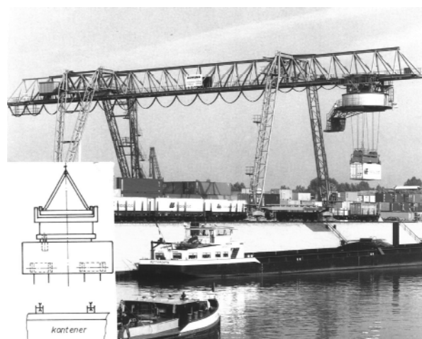
Figure 5. Lightweight structure of quay crane for river port terminals
