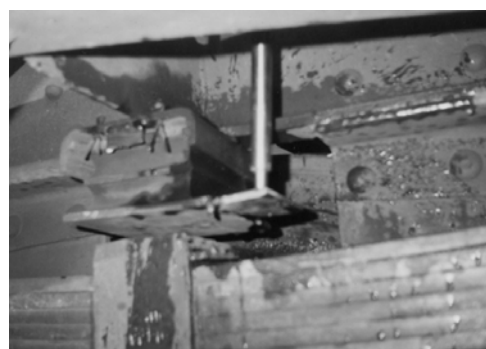
Figure 10. Operating tests of elastic rubber element in suspension system of "Fbd" wagon in TENT Obrenovac, Serbia
