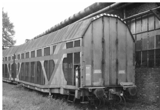
Figure 2. "Ddam" wagon used for car transportation (made in factory named "Bratstvo", Serbia)
