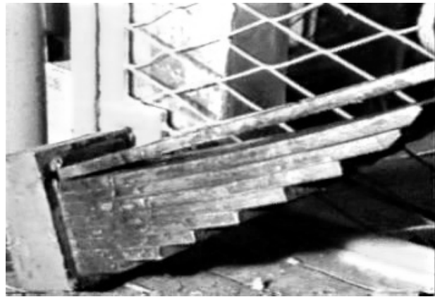
Figure 3. Laminated spring with cracked main leaf
