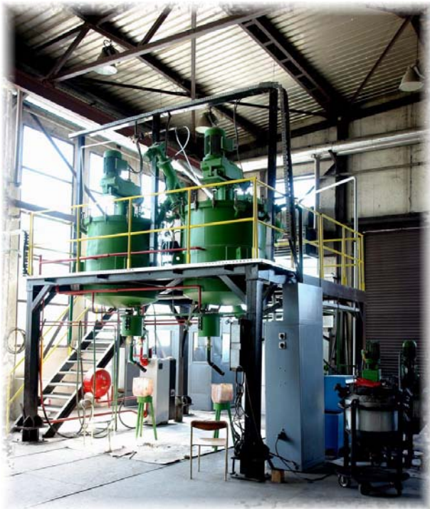
Figure 11. Technological line for preparation of mass and pressure casting of epoxy resin
