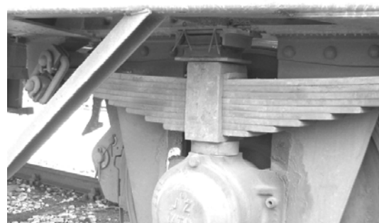
Figure 8. Elastic rubber element installed into suspension system of a "Fbd" wagon
