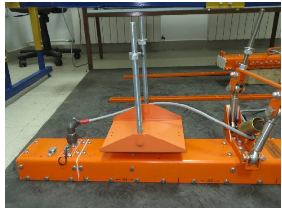
Figure 31: Specially designed support for the scanner
