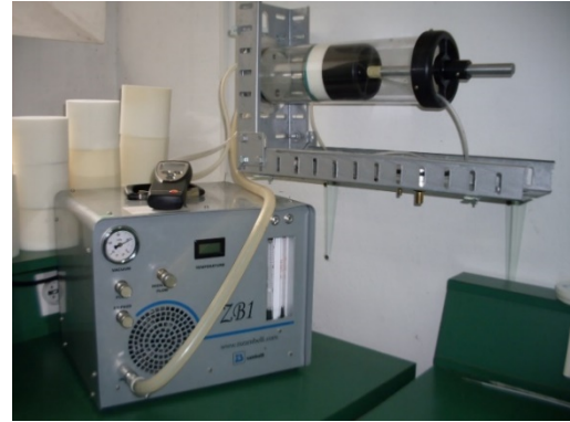
Figure 2: A view of the realized measurement system for determination of airflow resistance
