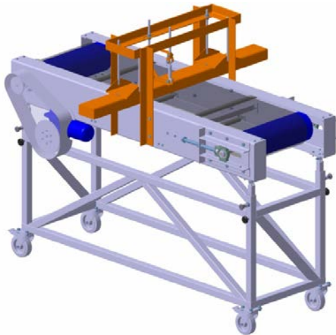
Figure 1: The 3D model of the test rig for NDT of steel cord belts
