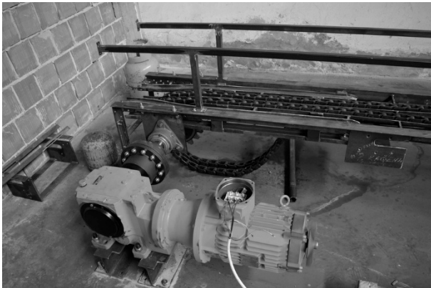
Figure 6: Connection of the motor and sprocket
