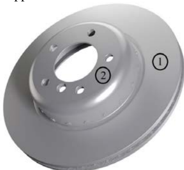
Figure 2: Two-piece brake discs 1-friction ring, 2-top hat [11]
