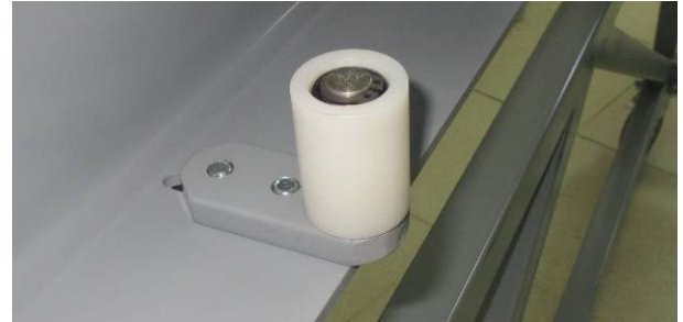
Figure 19: The training roller placed on the inner side of the belt conveyor frame
