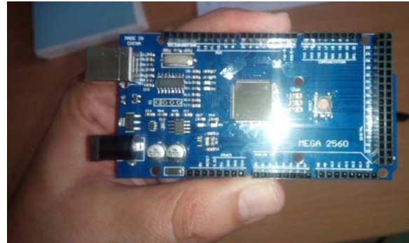
Figure 2: Single-board microcontroller Arduino
