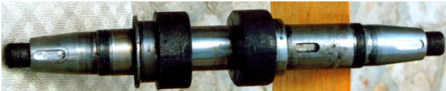
Figure 9: The appearance of the regenerated crankshaft of the motor ARAN
