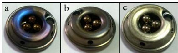
Fig. 6. Photographs of a mandrel after testing of oils: a – oil C; b – oil D; c – oil E.
