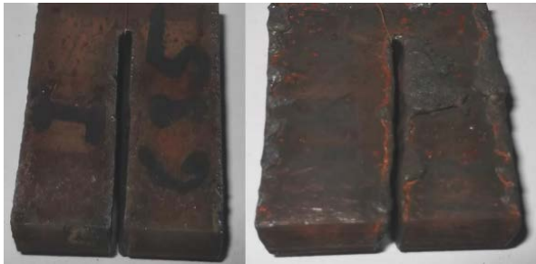
Fig. 5 Cutting with the First level of electrode wear and 635 mm/min (sample 3)
