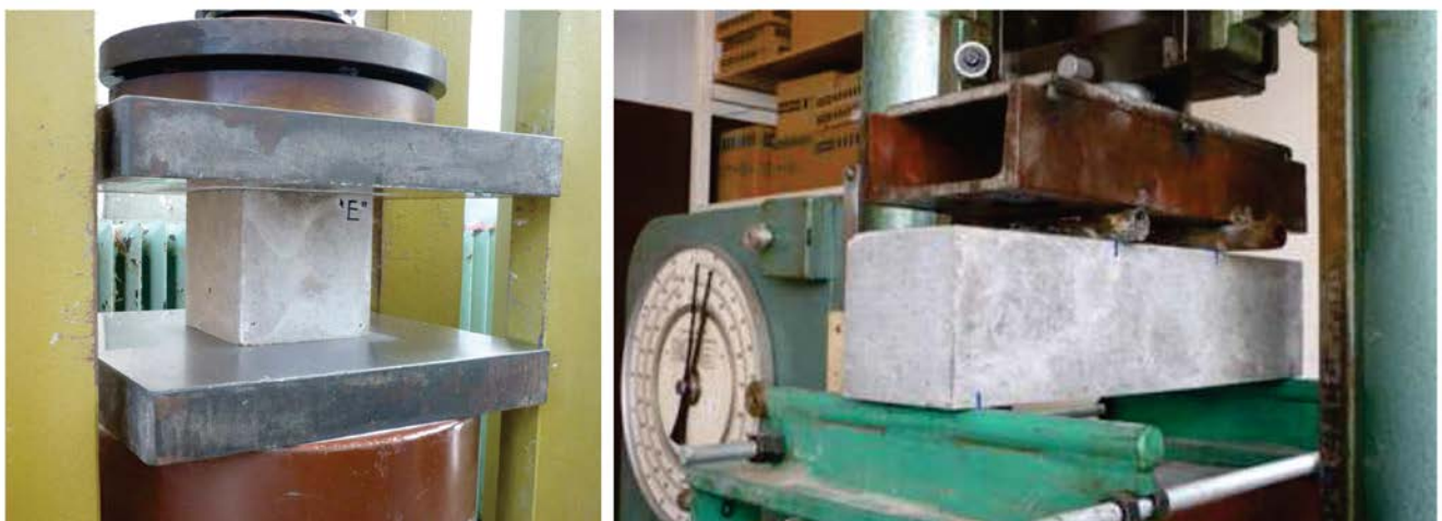
Figure 3: Testing of compressive strength (left); Testing of flexural strength (right)
