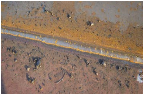
Figure 4. The visual appearance of self-shielded cored wire surface weld in a horizontal position
