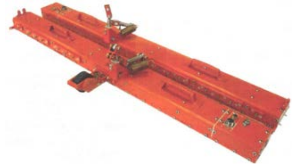
Figure 25: Disassembled modules of the Introcon S 2000 scanner (Courtesy of Intron)
