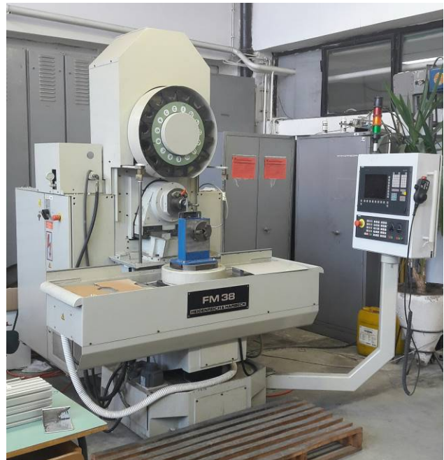
Figure 5: CNC Horizontal Center H&H FM38
