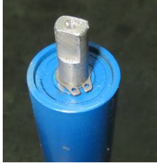
Figure 15. The belt conveyor roller's end
