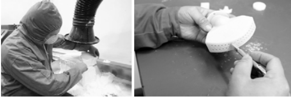
Figure 2: Removal of waste powder by machines (left) [9] and hand tools (right) [10]
