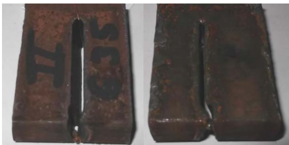
Fig. 8 Cutting with the Second level of electrode wear and 635 mm/min (sample 6)
