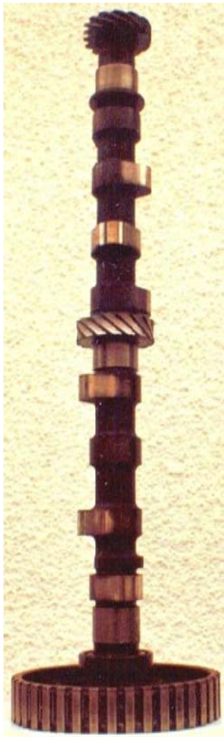
Figure 1: The damaged camshaft (the worn teeth of the gear in the middle)
