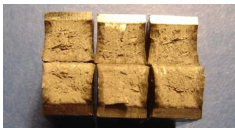
Figure 9. Appearance of the tubes fracture surface used in testing the toughness of weld
