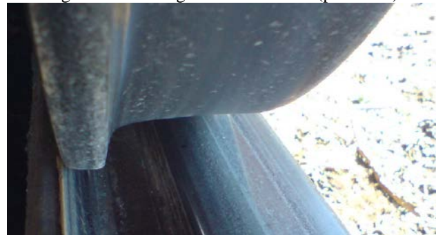
Picture 3: Contact of the non-working side of the flange with the flange of the inner rail.
