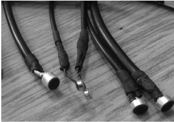
Figure 6: Microphones from the left to the right: 1) POM-5238L-R microphone from PROJECTS UNLIMITED and the other microphones from Kingstate Electronics Corp. 2) two KEEG1538WB-100LB and 3) two KECG2742TBL-A microphones
