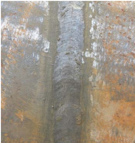
Figure 6. Surface appearance of joint test, welded with self-shielded cored wire, E71T-8 (Innershild NR 232)
