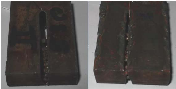
Fig. 6 Cutting with the Second level of electrode wear and 530 mm/min (sample 4)
