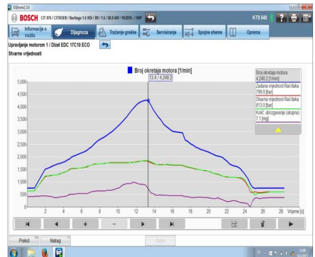
Figure 8. Diagram of set and actual values of pressure in the common rail system with continuous acceleration
