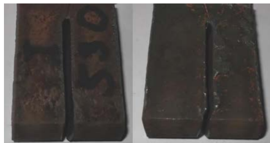
Fig. 3 Cutting with the First level of electrode wear and 530 mm/min (sample 1)
