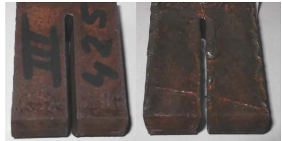
Fig. 10 Cutting with the Third level of electrode wear and 425 mm/min (sample 8)
