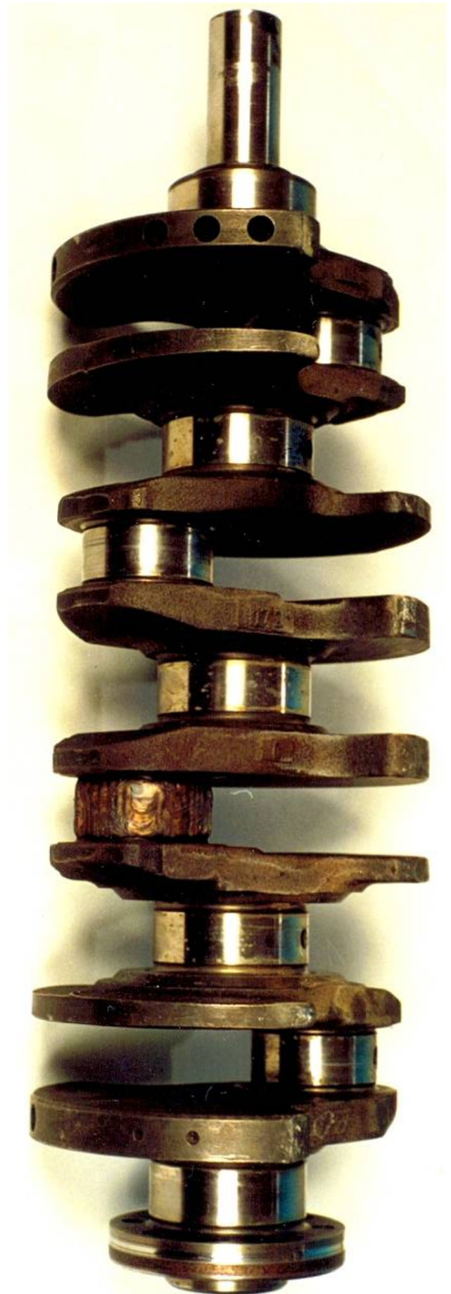
Figure 10: The appearance of the regenerated crankshaft of the motor VOLKSWAGEN (the hard faced journal is zoomed)
