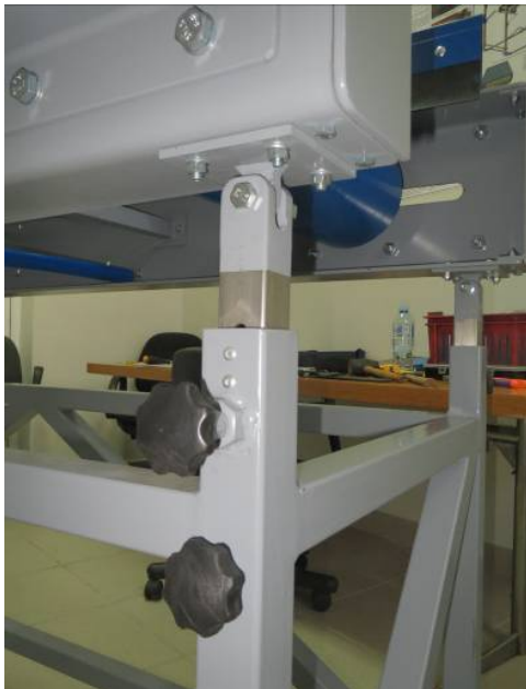
Figure 23: Levers for conveyor height and incline adjustment
