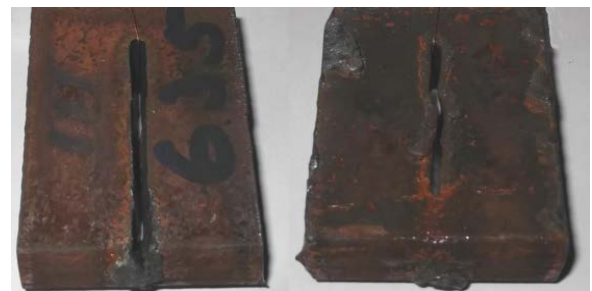
Fig. 11 Cutting with the Third level of electrode wear and 635 mm/min (sample 9)
