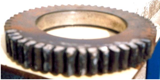
Figure 4: The appearance of the regenerated gear of the milling machine
