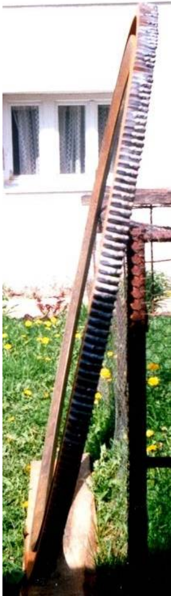
Figure 5: The damaged gear of the machine used for grinding stone in cement production
