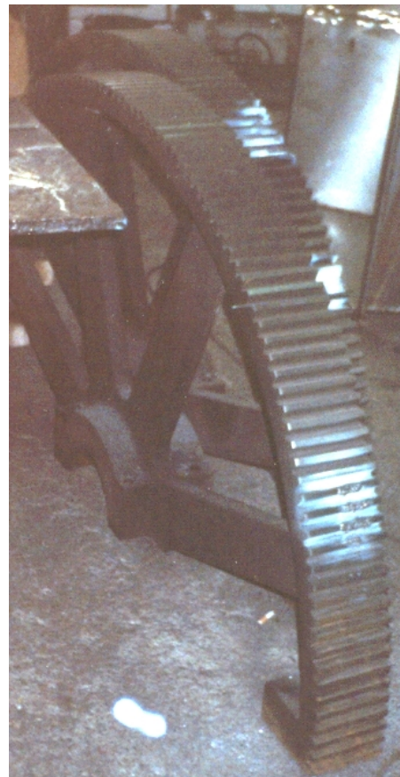
Figure 7: The appearance of the regenerated gear
