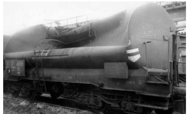
Figure 2: The deformed tank-wagon
