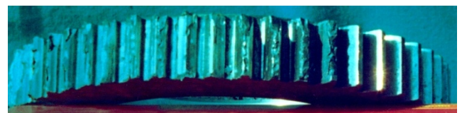
Figure 3: The damaged gear of the milling machine
