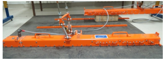
Figure 24: One scanner module consisted of 5 transducers
