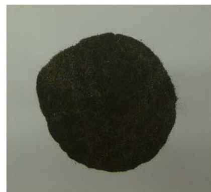
Figure 2: Appearance of copper flotation tailing
