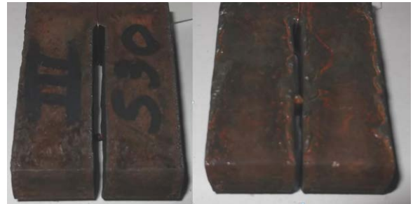
Fig. 9 Cutting with the Third level of electrode wear and 530 mm/min (sample 7)
