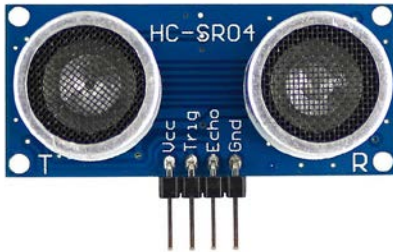
Figure 5: Ultrasonic sensor with pins
