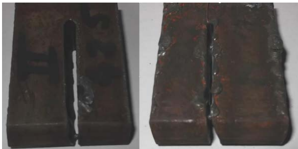
Fig. 7 Cutting with the Second level of electrode wear and 425 mm/min (sample 5)
