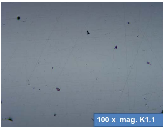
Figure 14. Test sample K1.1, material: steel 1.2709, polished with diamond paste 0.25 μm, magnification 100x
