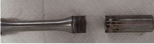
Figure 4: Unexpected failure at sample head
