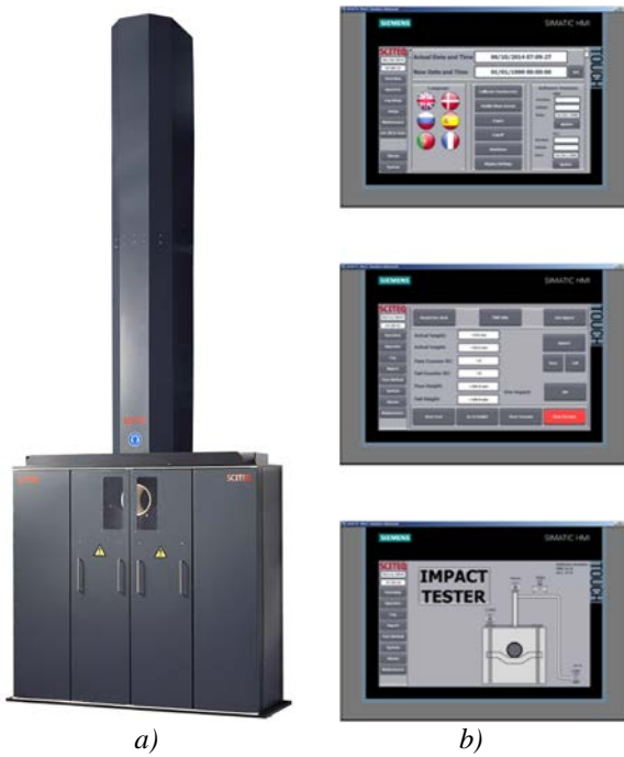
Figure 3: a) SCITEQ B50 Impact Tester; b) Interface of B50 [3]
