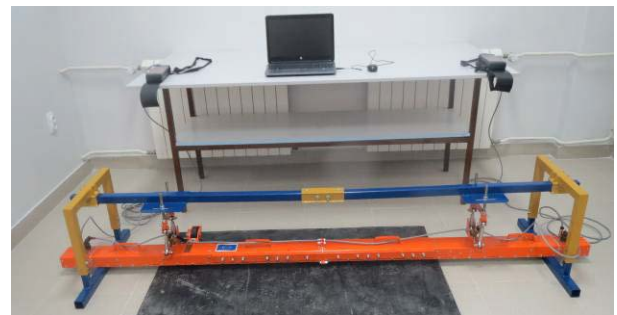
Figure 26: Assembled scanner with both modules fastened to each other with bolts and connected with cable
