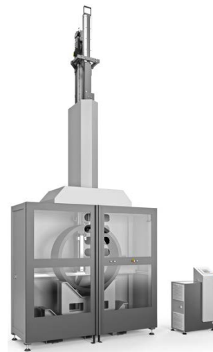
Figure 2: IPT Falling Weight Impact Tester Model no.1713 [2]
