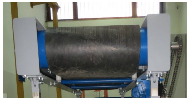
Figure 20: Training rollers in their working position adjusted for belt width of 400 mm
