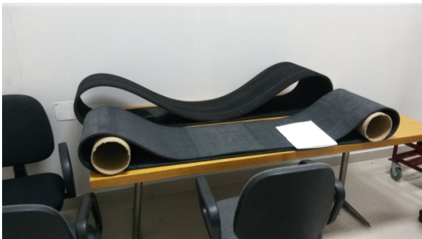
Figure 8: Steel cord belts for laboratory testing: worn-out belt (up) and specially made belt (down)
