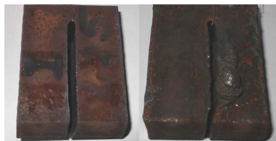
Fig. 4 Cutting with the First level of electrode wear and 425 mm/min (sample 2)
