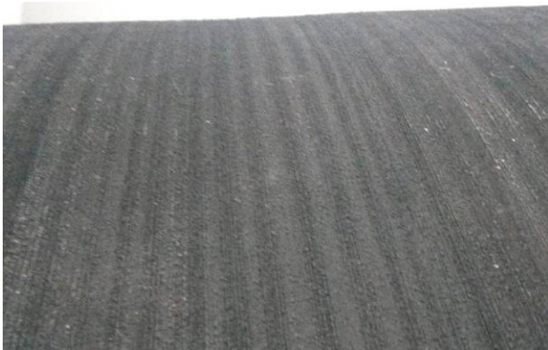
Figure 7: Textured surface of the worn-out steel cord belt
