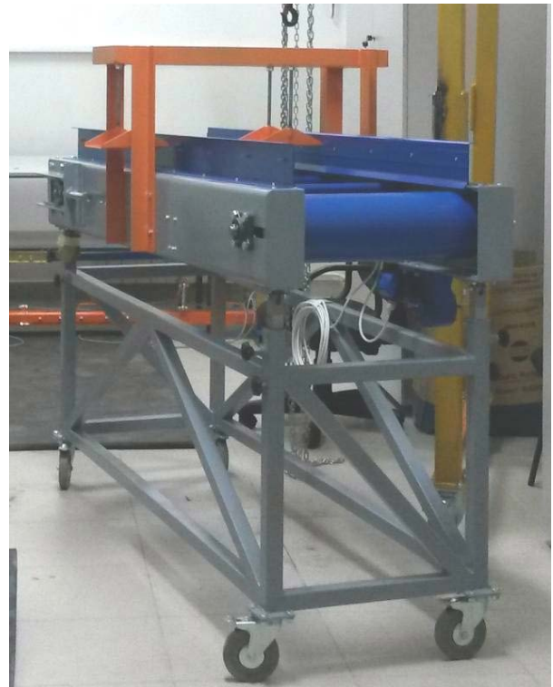
Figure 3: Produced belt conveyor, mounted on mobile carrier frame with scanner girder attached to its frame
